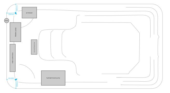
LOCATION FOR PRE-POWER THROUGH SLAB (power supply in conduit or flex to be installed in concrete slab at a MAXIMUM of 40mm above slab height)
