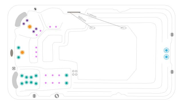
400 series jet 300 series jet 200 series jet volcano jet 7" cohuna jet swim jet neck jet air massage jet large divertor control small on/off control air control aromatherapy canister touchpad control filter box safety suction water return jet water spout
